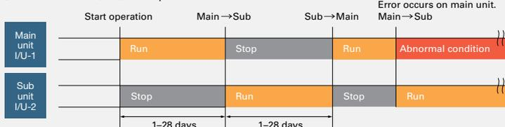
(Ex: When the request code is "313", each unit operates alternately in daily cycle.)
