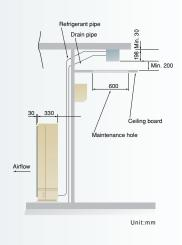
The branch box can be in-stalled inside above the ceiling.
