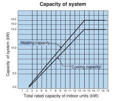
Note: Cooling capacity is based on; indoor temperature 27°CDB, 19.0°CVB, outdoor temperature 35°CDB. Heating capacity is based on; indoor temperature 20°CDB, outdoor temperature 7°CDB. The rated capacities above show the rise in the total indoor unit capacity when operating frequency is constant. Values for changes in capacity are fixed after accounting for variations in operating frequency and should be used as reference values.
