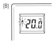
To turn the heater OFF press the OFF button for approximately 2-3 seconds.
