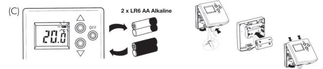
On the backing plate will be two AA Alkaline batteries. Remove the batteries and insert 2 new **AA Alkaline only** batteries, making sure the top battery is inserted first, then replace the front cover.
